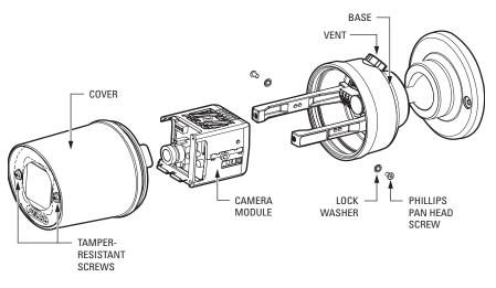
WARNING: To prevent damage to the camera or lens, the camera must be installed in the proper hole of the mounting bracket. If the camera is not installed in the correct hole, the window of the enclosure may be forced against the lens.
